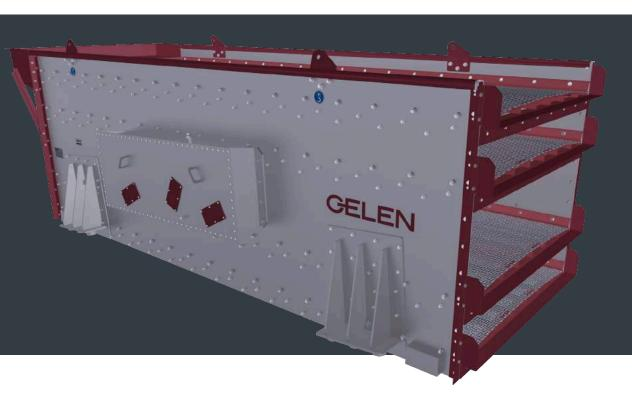
The ETE Series Elliptical vibrating screens are of horizontal type screens with triple shaft geared together resulting in elliptical motion which is the most efficient screening motion in the industry. The ability to change the shape and angle of the ellipse allows you to best suit your screening needs from scalping to fine screening. These screens are available in wet screening and washing applications.
